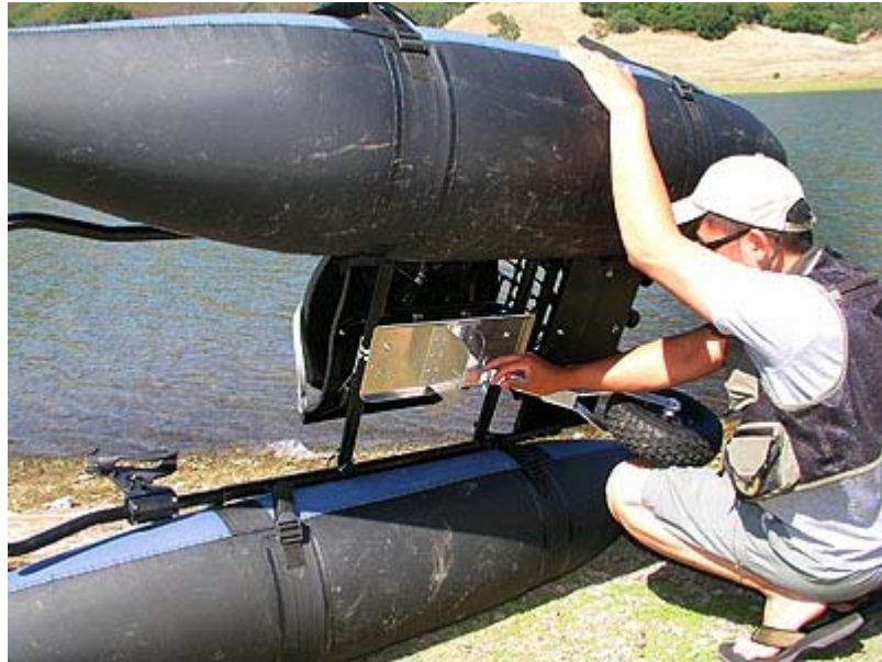
Before loading the pontoon you adjust the Launching Gear to it's open position
