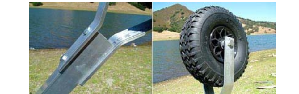
The wheel is reinforced and the actual wheel sports is a high quality rubber tire (30 PSI)
