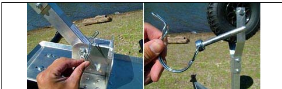
Adjusting the Launching Gear requires a quick pull and insert of the locking pin
