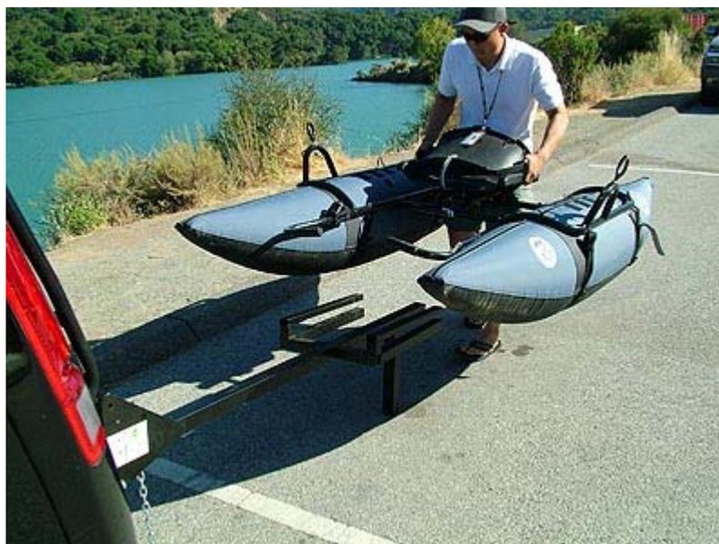
Lift the front of your pontoon boat and rest the crossbar beneath the seat on the center EZ Packer bar
