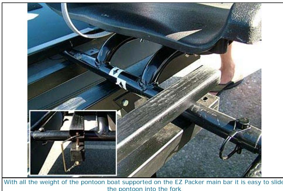
With all the weight of the pontoon boat supported on the EZ Packer main bar it is easy to slide the pontoon into the fork
