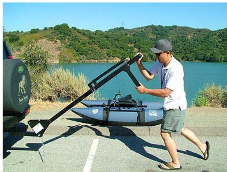
After removing the safety pin lower the EZ Packer into position on the ground
