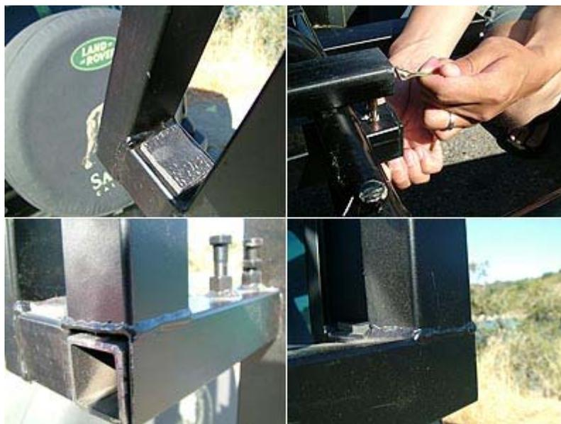
The EZ Packer is built with extremely sturdy steel and quality welds, powder coated for durability, and has numerous nice features like pads for pontoon protection, locking pins for ease of use and security
